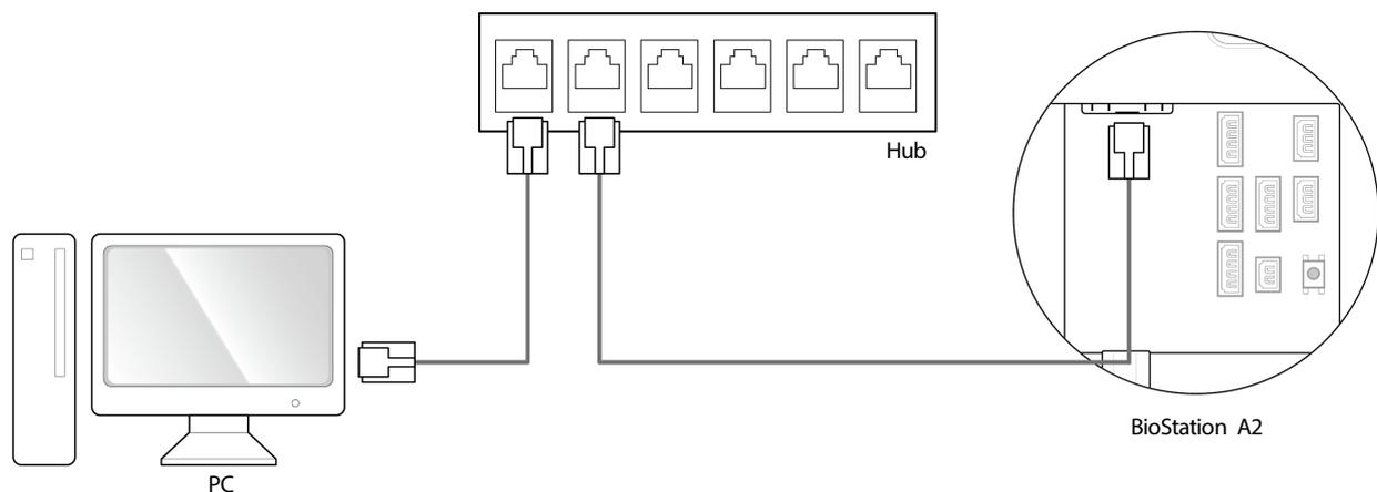
**LAN connection (connecting to a PC directly)**
